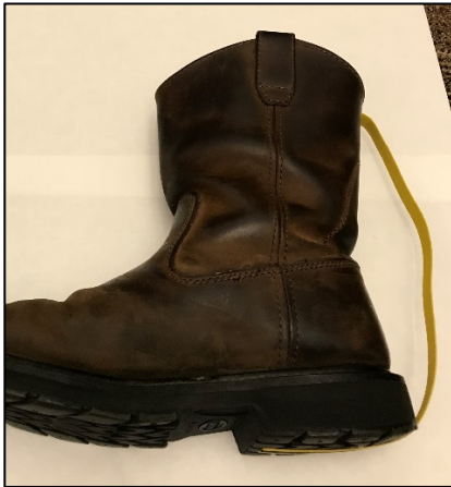
Figure VIII-3: Heel grounders. (Source: OSHA HRT)
