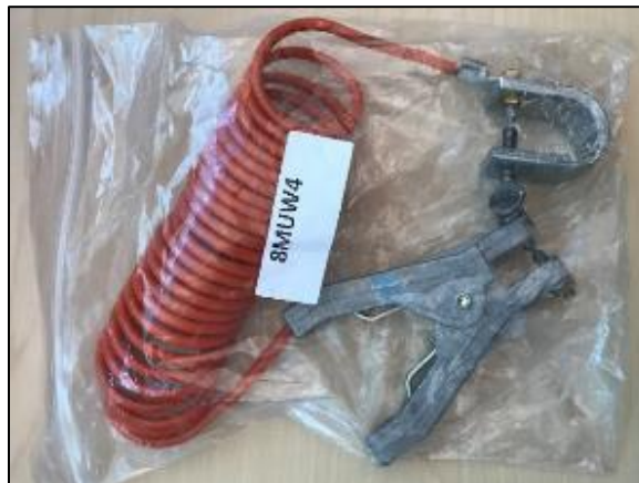
Figure VIII-2: Scoop bonding wire. (Source: OSHA HRT)
