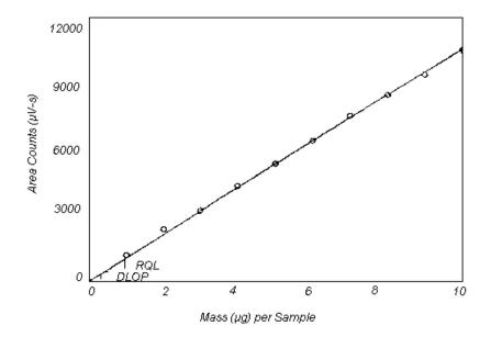
Figure 1.2.1. Plot of data to determine the DLOP/RQL.
