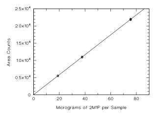
Figure 4.4.2. Instrument response to 2M1P. (Slope=290)
