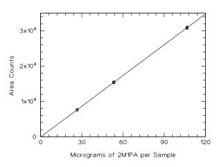
Figure 4.4.4. Instrument response to 2M1PA. (Slope=290)
