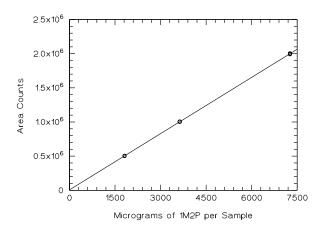
Figure 4.4.1. Instrument response to 1M2P. (Slope=275)
