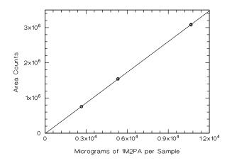
Figure 4.4.3. Instrument response to 1M2PA. (Slope=291)
