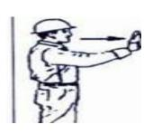
TRAVEL. Extend arm forward, hand open and slightly raised; make pushing motion in direction of travel.
