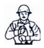
TRAVEL. (Both tracks). Use both fists in front of body, making a circlular motion about each other, indicating direction of travel, forward or backward( for land cranes only)
