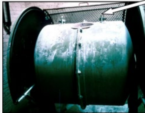
Interlocked guard on revolving drum
