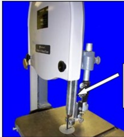
Bandsaw blade adjustable guard
