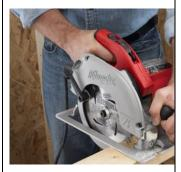
Tool users always need to check to make sure that all of the guards are in place if the tool has guards.
