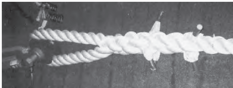
Figure D-017 Properly Made 3-Strand Eye Splice (correctly made – shown for reference)
