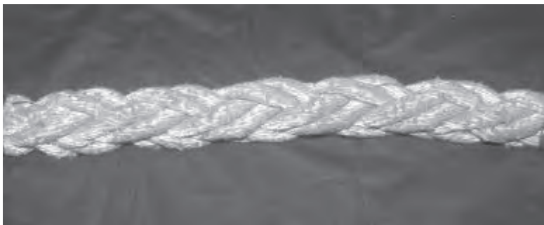
Figure 2 8-Strand Plaited Rope
