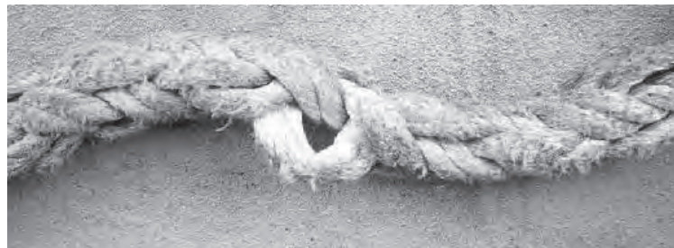
Figure D-013 Pulled Strand in 8 Strand Rope
