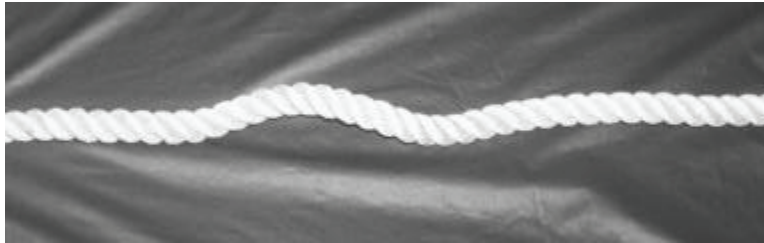
Figure D-024 Corkscrew Due to Twist
