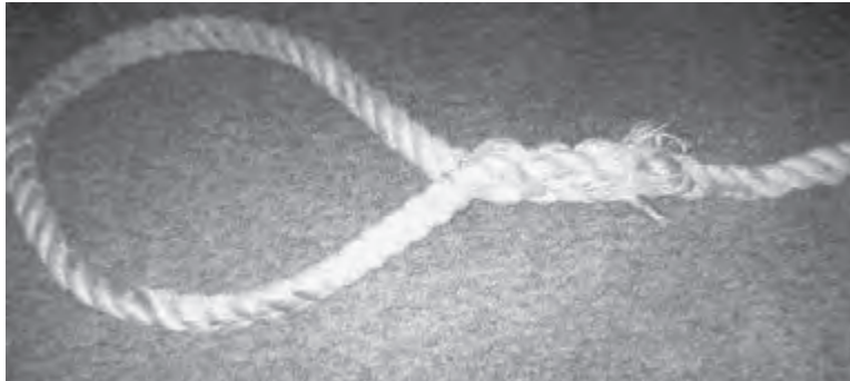
Figure D-018 3-Strand Splice of Poor Quality
