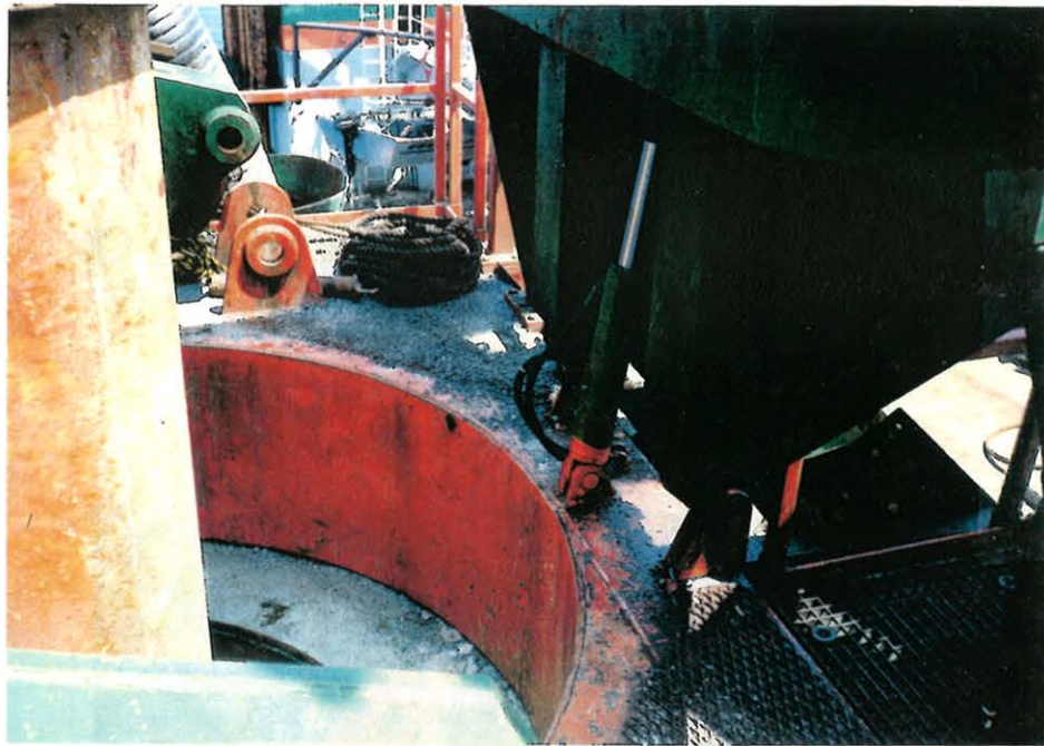
Figure 3-10 Lower Side of the Platform Door with the Repaired Hydraulic Jack.
