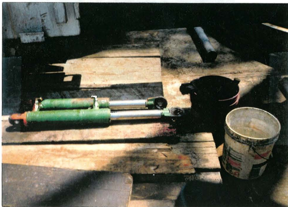
Figure 3-11 Two Damaged Hydraulic Jacks as a Result of the Accident.
