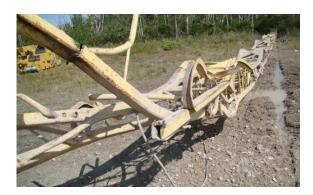
Figure 10 – Lower Sections of Gin Pole
