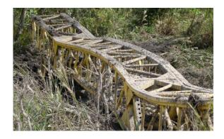
Figure 14 – Gin Pole Section Break
