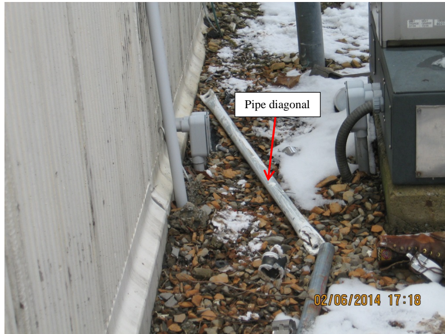
Figure 3. The fourth round diagonal, removed earlier from the tower, was found on the passageway near the tower.
