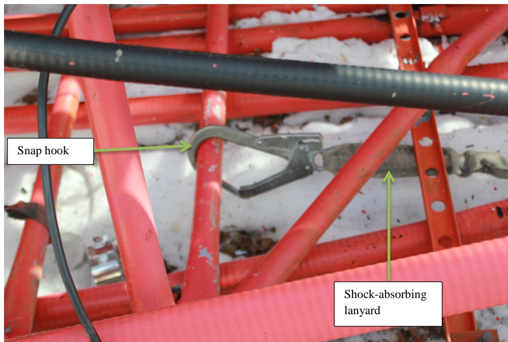
Figure 17. The snap hook from one of the injured employees was anchored to a horizontal bracing member of the tower (WVSP Photo 5969).
