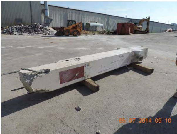
Fig. 102 NE corner column showing inadequate lap splice
