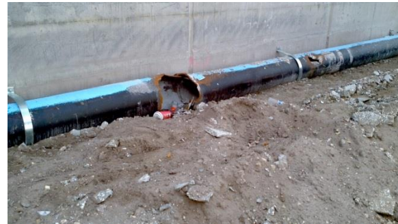
Fig. 20 Fractured 12" Water pipe
