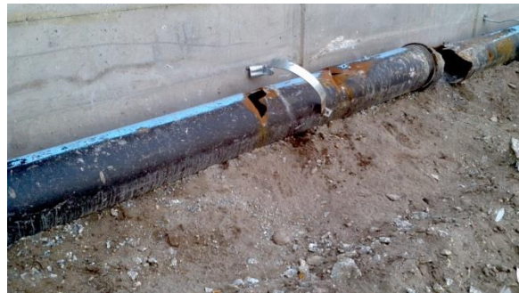
Fig. 18 Fractured 12" Water pipe
