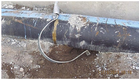
Fig. 17 Failed clamp for water pipe
