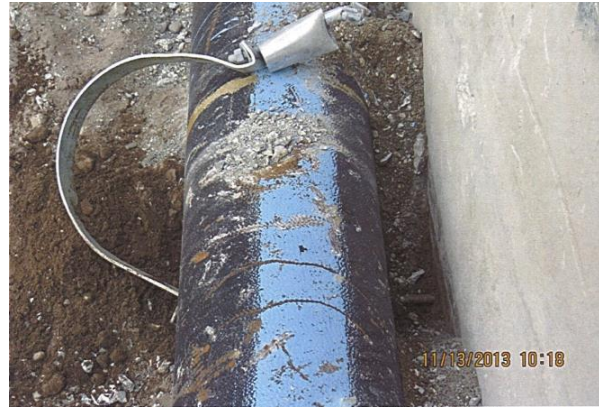
Fig. 16 Failed clamp for water pipe
