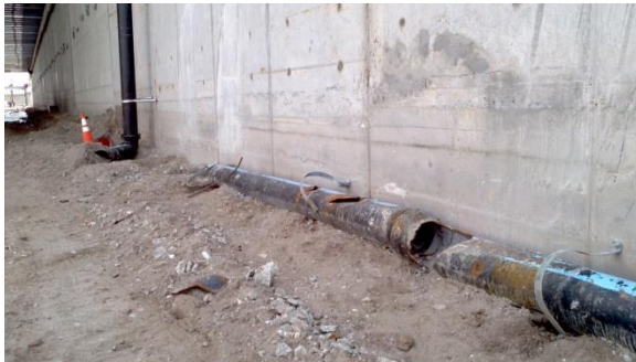
Fig. 19 Fractured 12" Water pipe
