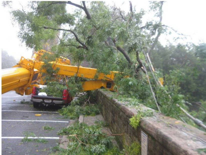
Figure 13. Another Parked Red Truck Damaged by the TY Guys of the Telescopic Boom (Taken from KCE Structural Engineers, PC).
