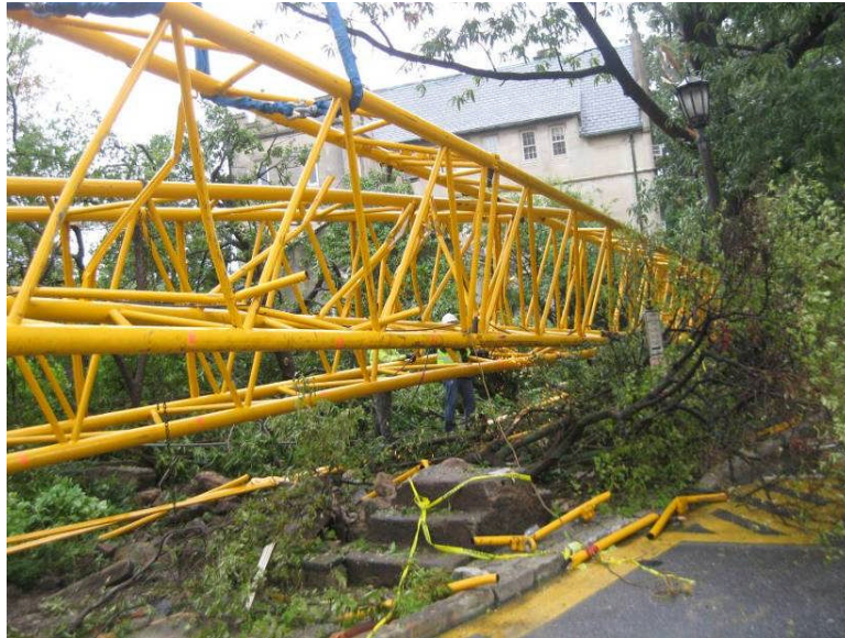
Figure 10. Broken Lattice Jib Pieces after the Collapse (Taken from KCE Structural Engineers, PC).
