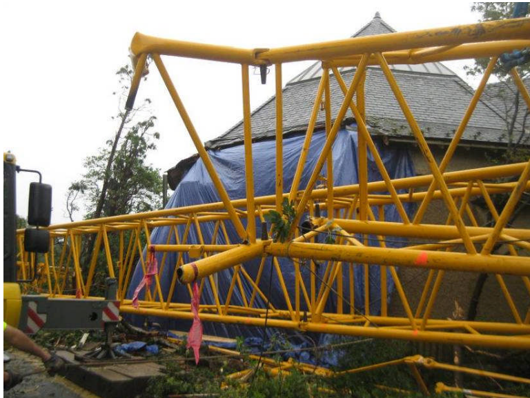
Figure 11. Herb Cottage Damaged by the Lattice Jib (Taken from KCE Structural Engineers, PC).
