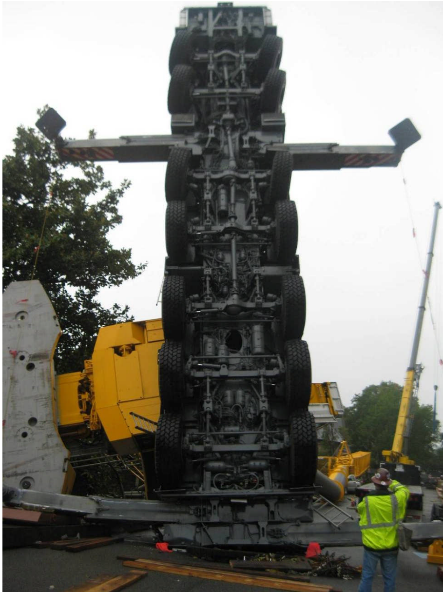
Figure 14. A Near Vertical Position of the Carrier and the Superstructure after the Collapse (Modified from KCE Structural Engineers, PC).
