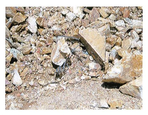
Figure 20 Type and Size of Rock Pieces at the Center of the Collapse.
